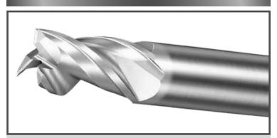
3-Flute design for aluminum allowing for both heavy profile and slotting applications. Advanced cutter geometry with wiper flats for improved floor finish. Available coated and uncoated.
