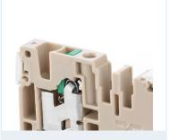
The terminal blocks are delivered with pre-loaded springs. The switching status of the pre-loaded contact point is signaled by the position of the pusher.
