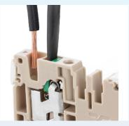
The pusher can be pressed to release the conductor quickly and easily at any time, preloading the contact point for further wiring.
