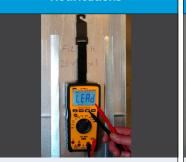
Multimeters that measure current have a Lead Warning and Fuse Blown notifications that prevent the end-user from using the meter with the leads in the wrong ports and notifies them when a fuse is blown.
