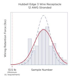
Compared to the UL minimum requirement for wire retention, EdgeConnect screwless termination offers superior strength.
