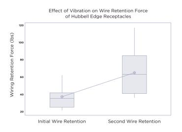
Upon installation, a 10 AWG THHN stranded wire required 40 lbs of force to disengage. After exposure to vibration per the UL standard, 65 lbs of force were required to disengage.
