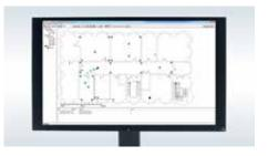
The Locating Manager is a software position of the individual transponders and passes the details on to the higher level systems via defined interfaces.
