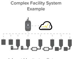
1 Asset Monitoring Gateway 2 Vibration Sensors 2 Current Transformers 2 Pressure Sensors 2 Vib. and Temp. Sensors
